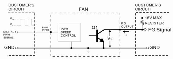
\*TRANSISTOR Q1 AT "ON" POSITION
