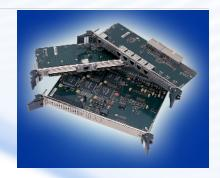
Our CP6900 is an unmanaged, low cost 10/100 Ethernet switching platform. It offers 24 10/100 auto negotiating Ethernet ports in a rugged, hot-swap, CompactPCI® 6U form factor. The result is a cost-effective switching solution for OEMs & integrators looking to quickly launch carrier-grade IP products with basic Ethernet switching capabilities.
