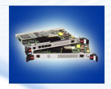
The CP6922 is an embedded Ethernet switch compatible with both standard CompactPCI® and PICMG® 2.16 backplanes. It is designed to be used as a high-speed interconnect within server blade chassis or as a core switch in fault-tolerant clusters of embedded systems.
