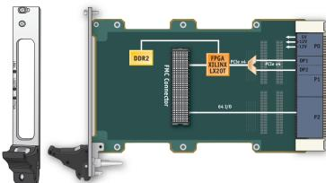
Kontron also offers a development kit containing: FMC-SERO a sample FMC with wrapping areas, a simple FPGA IP and a Linux rpm with drivers, utilities and test programs. This kit allows non regression tests and is the base for customized derivative work.
