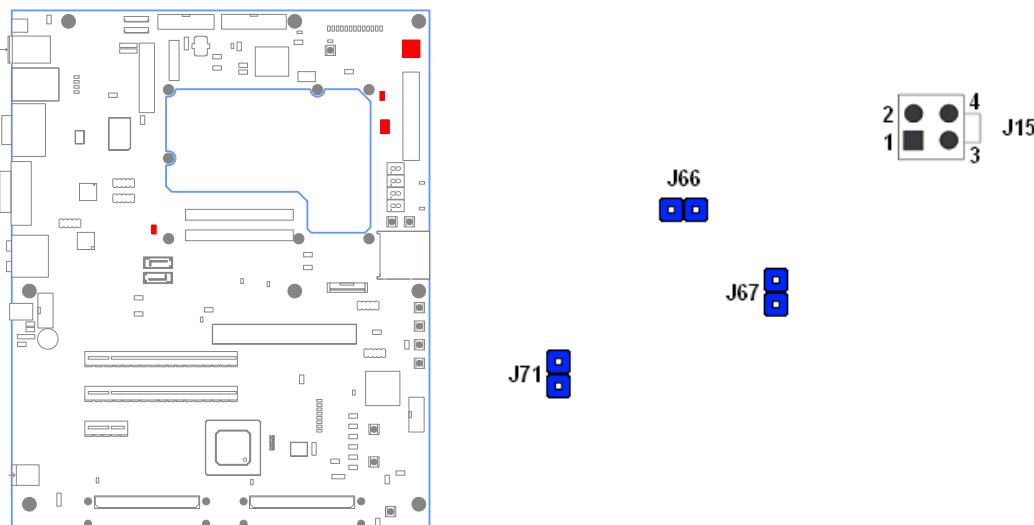
Additionally Kontron modules support single supply operation without standby voltage. To enable module single supply mode open jumper:
