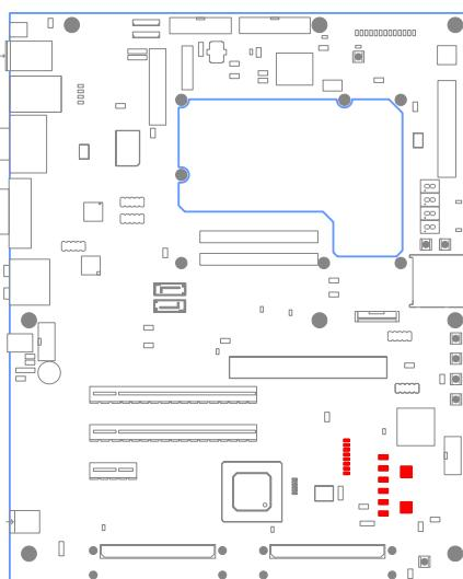
For debug purposes, LEDs and GPIOs are connected to FPGA. 2 of GPIOs are also connected to buttons. For GPIO use, ensure FPGA internal pull-up is enabled. LEDs and GPIOs are connected to FPGA banks 3, 4 and 5.
