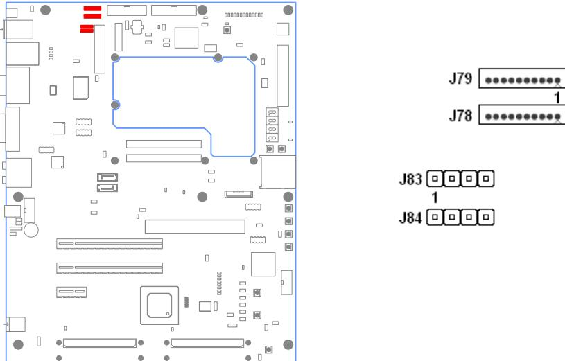
J78 and J79 allow both interfaces to be used as 2-pin RS232 interfaces COMA and COMB with Kontron Adapter cable [KAB-DSUB9-2](#). Please check the documentation of your module if this interface is supported and how to configure.
