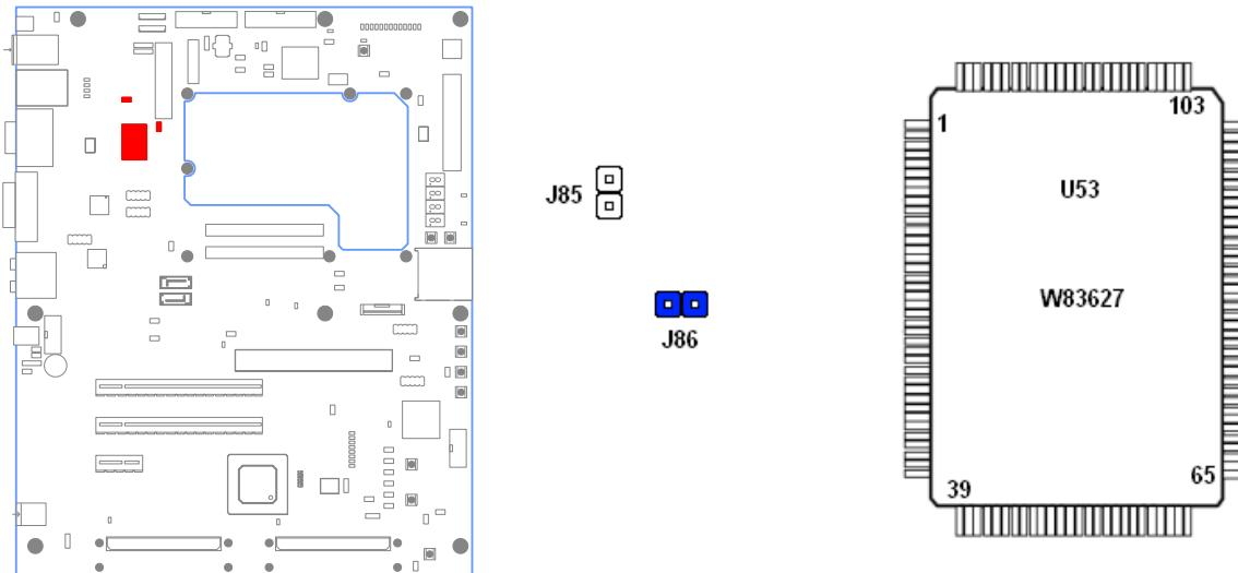
The configuration jumpers J85 enables the SIO keyboard controller when closed. Open J86 to hold the Super-I/O in reset to simulate a legacy free backplane.
