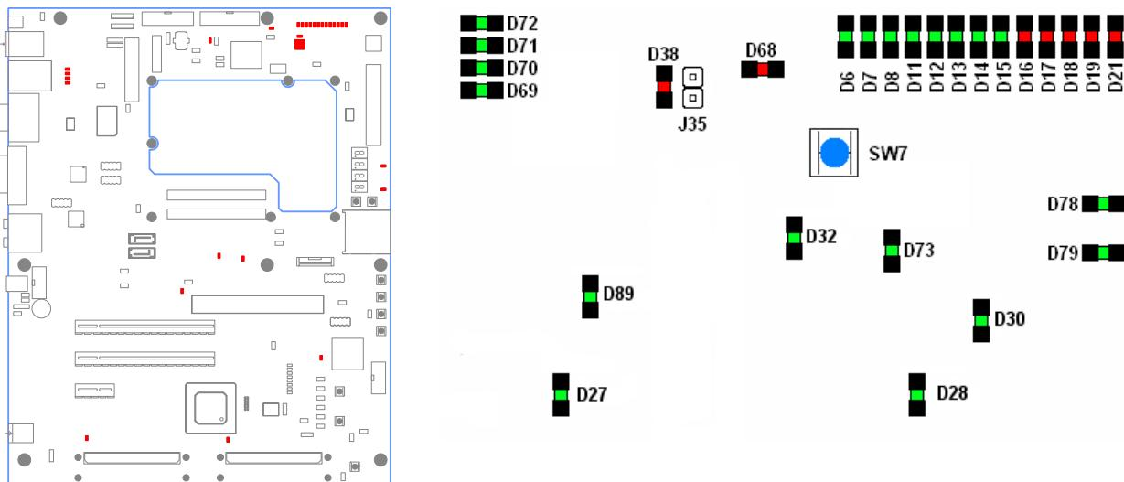
A front panel HDD LED can be connected HDD Activity connector J35. D68 indicates an active watchdog trigger WDT. The output is buffered and the switch SW7 resets the Latch. LEDs D27 and D28 indicates the presence of HSMC cards.
