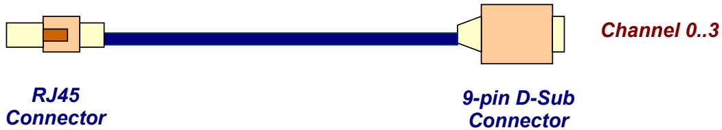
Figure 5-5: Four-Channel Front Panel Adapter
