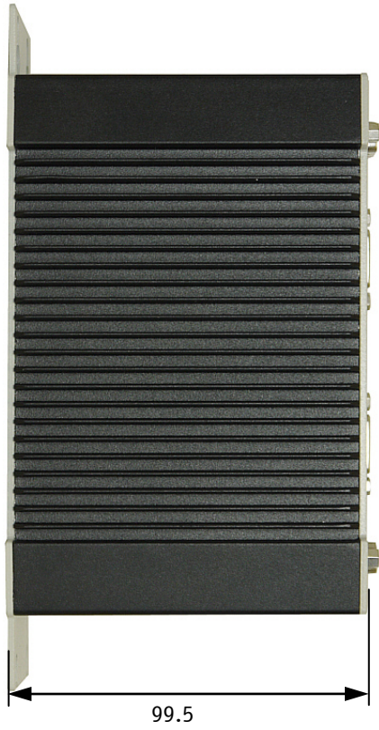
Fig. 24: Dimensions: left side
