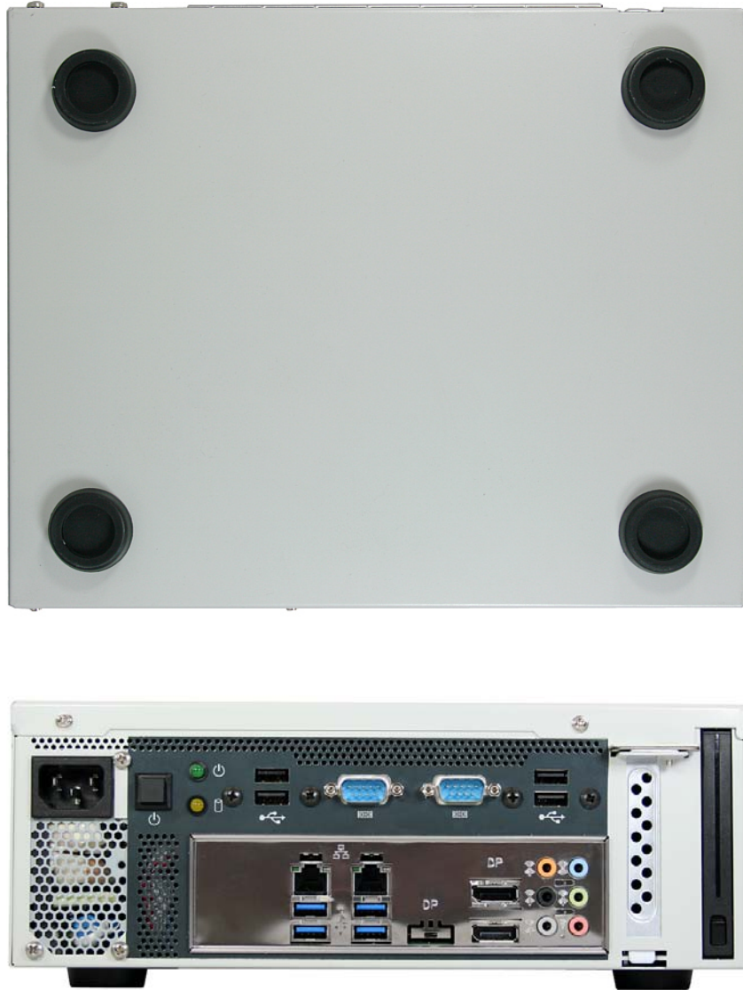
Fig. 19: Desktop version of the KBox B-101, with rubber feet attached
