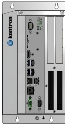
Fig. 8: Front side view config. with removable drives
