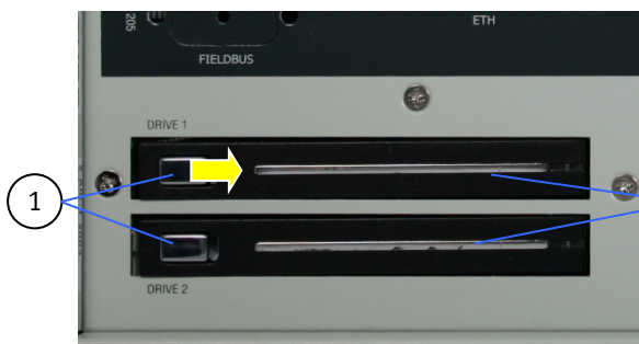
Fig. 25: Drive 1 and Drive 2 for removable 2.5" SATA HDD/SSD (option); closed drive bays
