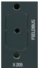
Fig. 23: X 205 – Location for the optional FIELDBUS interface
