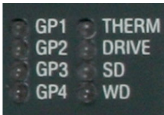
Fig. 22: Detail - Status and General Purpose LEDs
