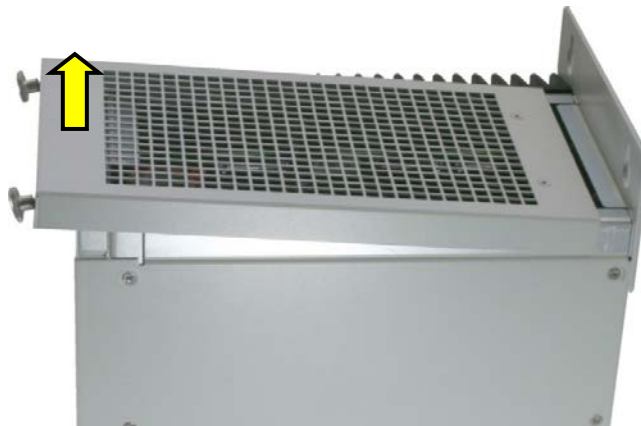
Fig. 39: Removing the cover (detail of the KBox C-101-2)
