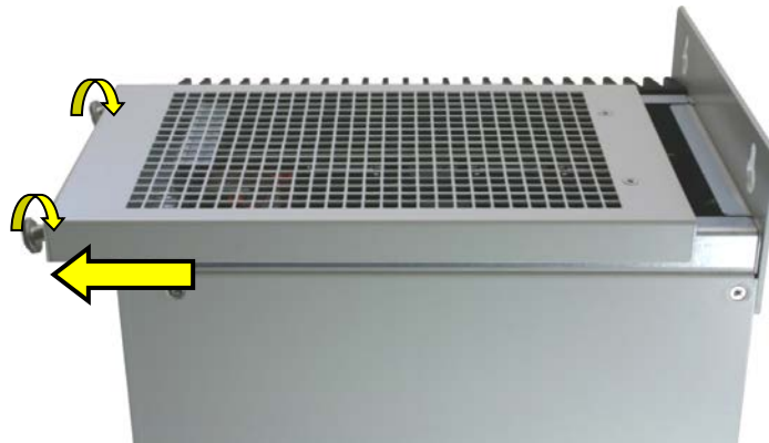
Fig. 38: This movement allows you to remove the centering and fixing bracket of the top cover (detail of the KBox C-101-2)
