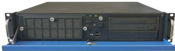
Fig. 4: Rackmount version with opened access door
