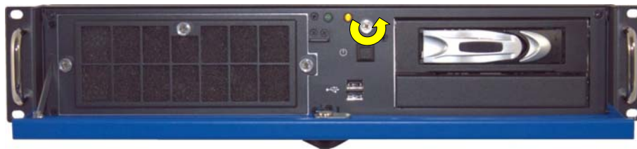
Fig. 32: Loosen the cover fastening knurled screw on the front side
