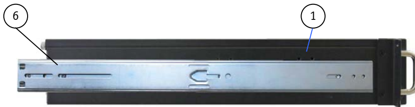
Fig. 51: KISS 2U V2 platform with slide rail in pushed-in position
