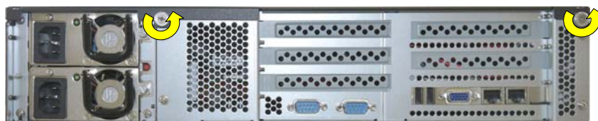
Fig. 33: Loosen the knurled screw on the rear side
