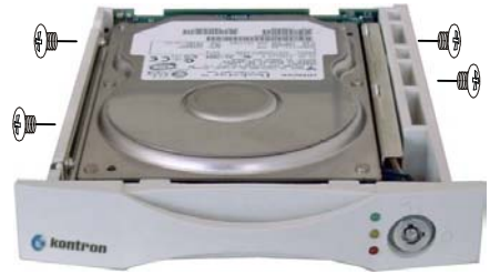
Fig. 12c: SATA HDD securing – Step 3
