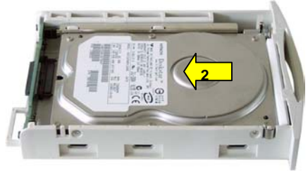
Fig. 12a: SATA HDD installation – Step 2
