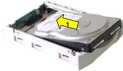
Fig. 12: SATA HDD installation – Step 1
