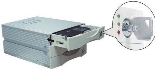
Fig. 13: Drives cage assembling
