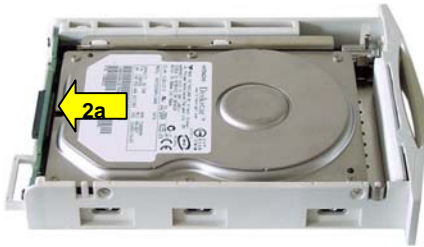
Fig. 12b: SATA HDD installation – Step 2
