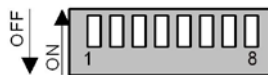
Fig. 27: Onboard DIP-Switch (SW1) with DP1 up to DP8 for RS422/RS485 serial communication settings
