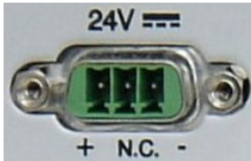
Fig. 21: Detail of the DC Power connector shown without Phoenix terminal
