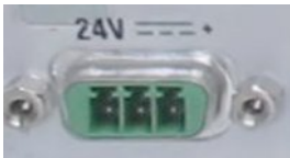
Fig. 14: DC Power connector on the bottom (rear) side of the Medi Client IIA system
