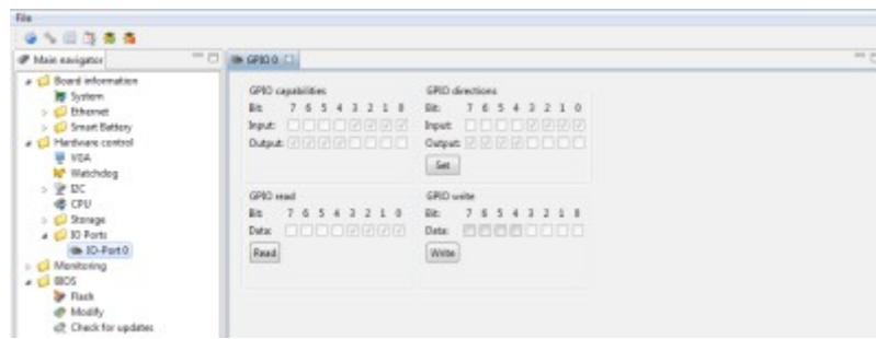
The GPI and GPO pins can be configured via JIDA32/K-Station. Please refer to the JIDA32/K-Station manual in the driver download packet on our [customer section](#).
