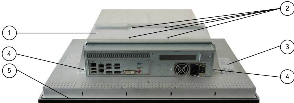
Fig. 37: OmniClient with U-shaped VESA 100 adapter (shown mounted to a HMI-OC215)
