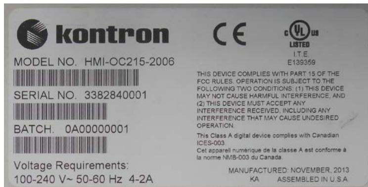
Fig. 1: OmniClient type label (shown as type label for a HMI-OC215 system, AC configuration)
