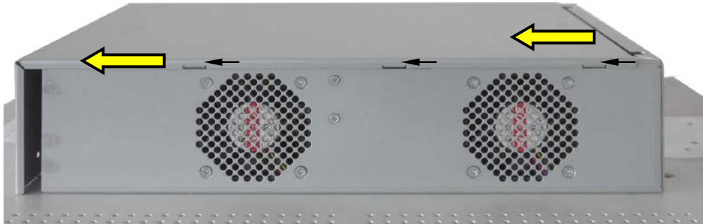
Fig. 29: Detail of OmniClient - Pull out the cover of the computer base
