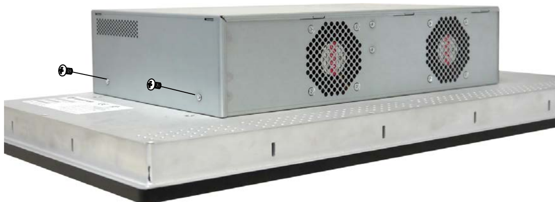
Fig. 28: Detail of OmniClient – Removing the screws that secure the cover of the computer base
