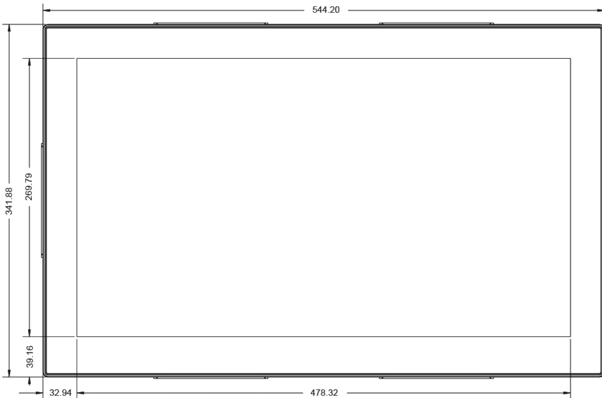
Fig. 24: Mechanical specification - Front view of an HMI-OV215
