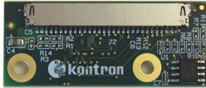
Figure 8. KLAS Board 43mm x 18mm
