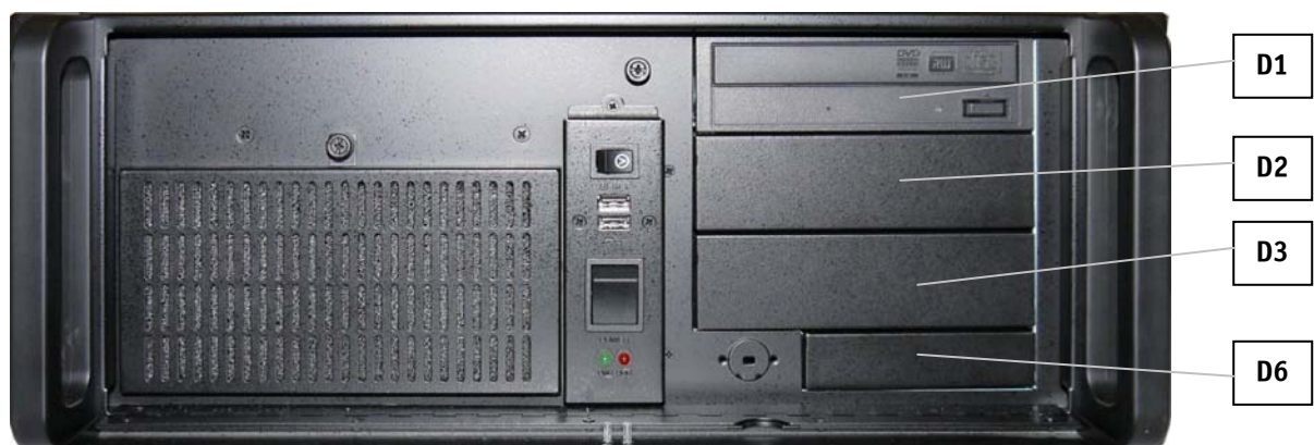
Fig. 11: Front accessible drive bays (e.g. D1 equipped with a DVD drive)
