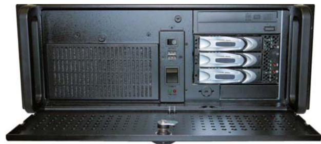
Fig. 3: VRack 4U - configuration with DVD and DA435 drives
