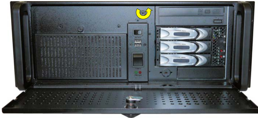
Fig. 17: Loosening the knurled cover fastening screw on the front side
