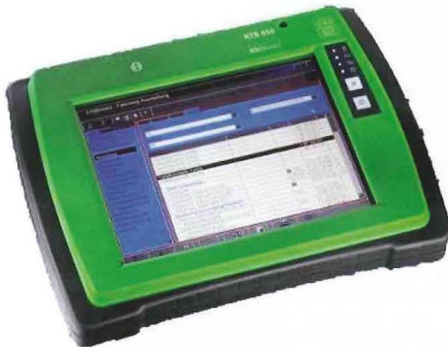
Figure 2: With the help of Kontron MARS, mobile applications — such as the diagnostic system for automobiles shown here — can be supplied with uninterrupted energy: A fall back battery allows to replace the discharged battery without intermission.
